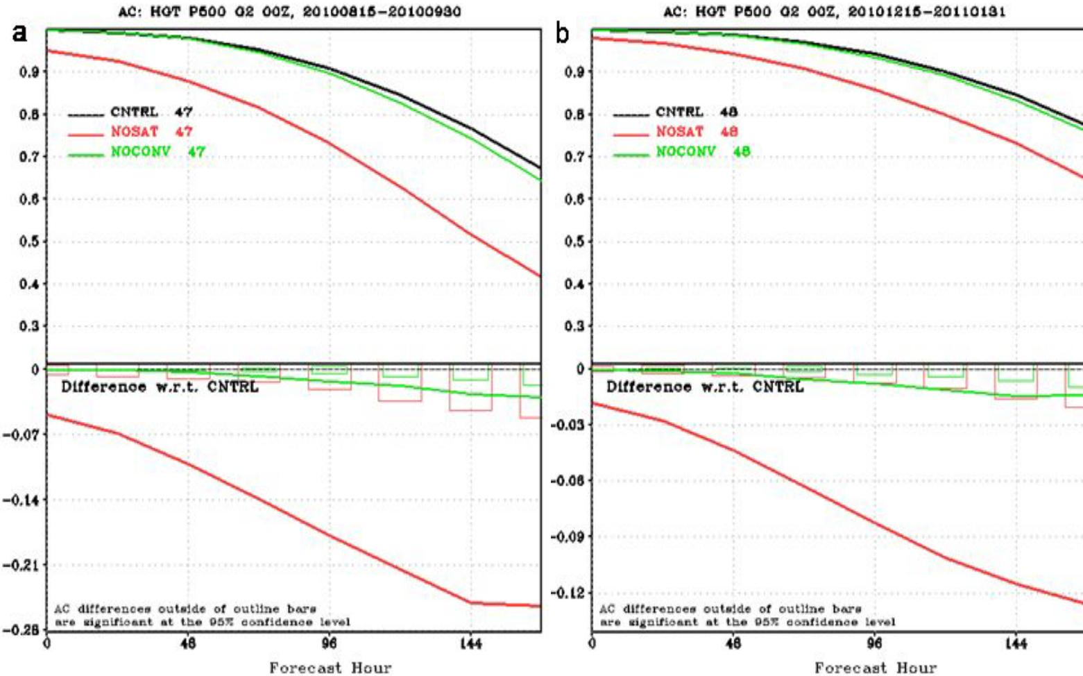
**Figure 1** Analysis through day 7 die off curves of anomaly correlations for geopotential heights during (a) August – September 2010 and (b) December 2010 – January 2011. The Control is in black, the no satellite data experiment is in red and the no conventional data experiment is in green. The lower panel curves are differences with respect to the control. Lines outside the same color box are statistically significant at the 95% level.
