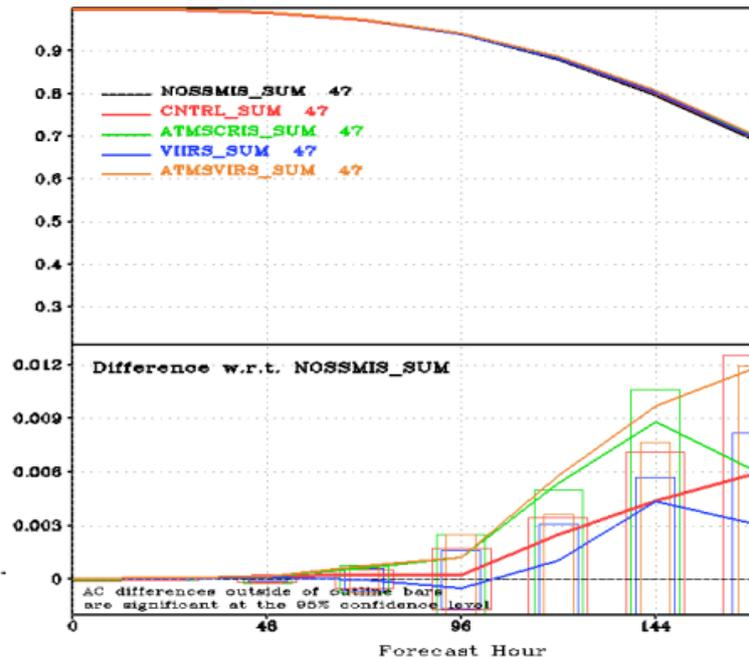
Global impacts on 500 hPa geopotential height anomaly correlation (AC), for forecasts valid at (above left) 00Z, (above right) 06Z, (below left) 12Z, and (below right) 18Z. Upper portions of each diagram represent the AC for each experimental run; lower portions are the differences in AC with respect to the NO SSM/IS (no early morning satellite) forecasts. AC differences outside of their corresponding color bars are significant at the 95% confidence level.
